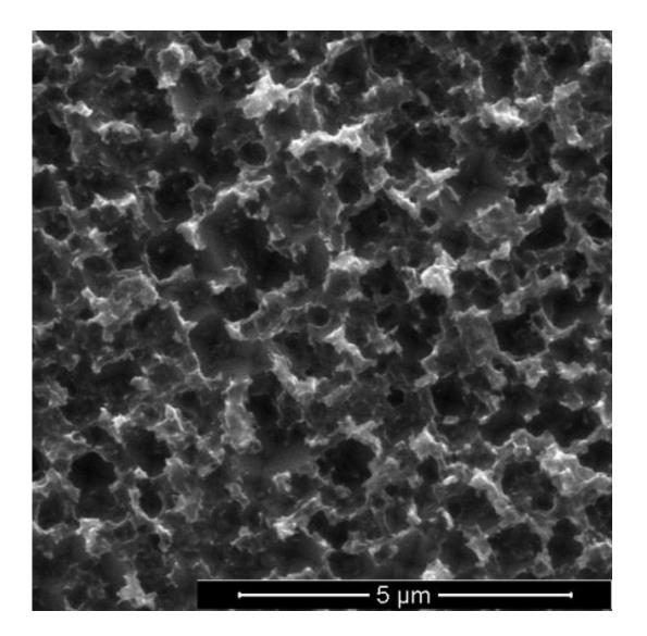
Rice University scientists have reduced to one step the process to turn silicon wafers into the black silicon used in solar cells. The advance could cut costs associated with the production of solar cells. Here, a top-down view shows pyramid-shaped pores etched into silicon over eight hours. Credit: Barron Group/Rice University
