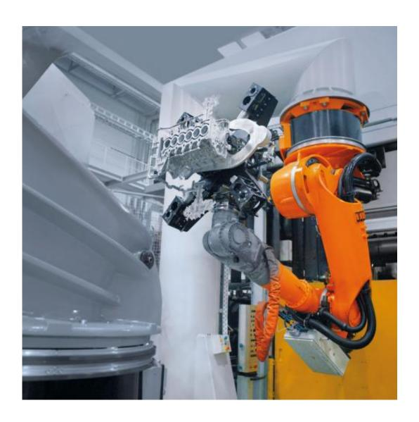
Siemens wants to further reduce the power consumption of manufacturing robots in the automotive industry. One approach to this problems deals with movement patterns that require less acceleration energy. Working with Volkswagen and Fraunhofer Gesellschaft as part of the Green Carbody Technologies (InnoCaT)
