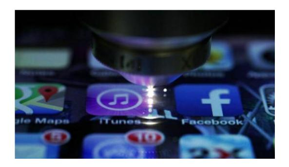
An invisible waveguide (pathway for light) being written via laser into a smartphone's display glass is shown. The waveguide is a horizontal line from the left side of the screen, but it cannot be seen with the naked eye. Credit: Optics Express
