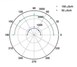
Figure 4: The angular response of the iPhone 4S smartphone at two different dose rates,  $50 \,\mu\text{Sv/h}$  and  $150 \,\mu\text{Sv/h}$ . The dots represent the number of counts recorded by the phone at different orientation angles.
