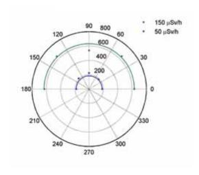
Figure 3: The angular response of the Samsung Galaxy S2 smartphone at two different dose rates,  $50 \,\mu\text{Sv/h}$  and  $150 \,\mu\text{Sv/h}$ . The dots represent the number of counts recorded by the phone at different orientation angles.
