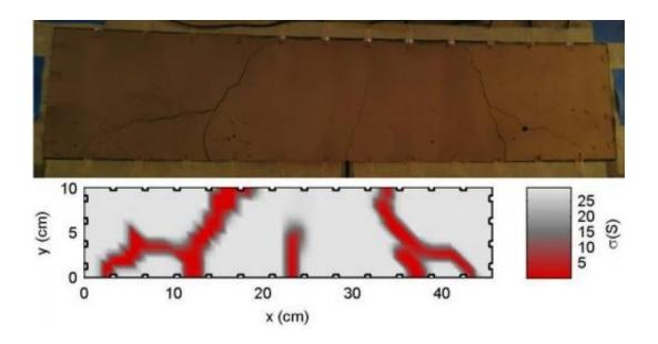
The "sensing skin" technology detects cracks in concrete (as in top image) and reports when and where the damage took place (as in bottom image). Click to enlarge. Credit: Aku Seppänen
