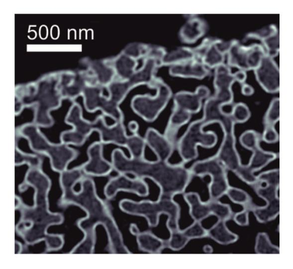
A cross-section of the tomograph of the glass sample studied. The glass contains
