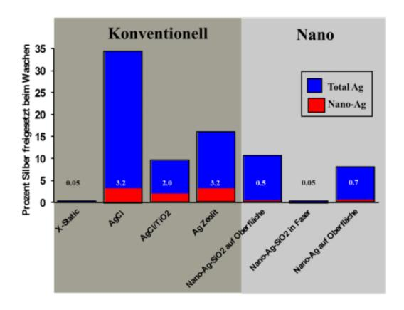
This graph represents the percentage of silver coating that is washed out during a laundry cycle (blue) and percentage of nano-particles (red). Textiles coated with nano-silver release fewer nano-particles than those with conventional coatings. Credit: Empa
