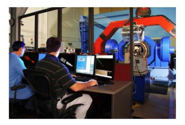
The Georgia Tech Research Institute (GTRI) is helping improve hardware-in-theloop simulations, which use portions of real missile hardware -- with any missing pieces made up by simulated components -- to test fire missiles.
