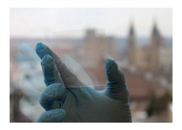
A transparent layer of electrodes on a polymer surface could be extraordinarily tough and flexible, withstanding repeated scotch tape peeling and bending tests, providing for a shatterproof smartphone touchscreen. Credit: The University of Akron
