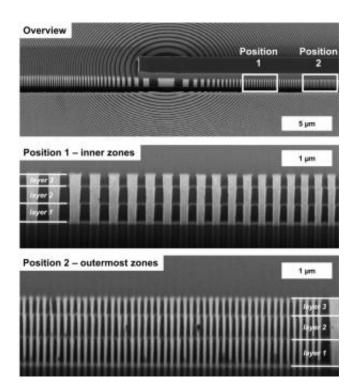
These scanning electron micrographs show how accurately the three Fresnel zone plates were positioned above one another. 3D X-ray optics of this kind allow the resolutions and optical intensities to be considerably improved. Credit: S. Werner/HZB
