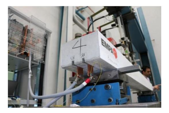
A concrete beam, which was reinforced with two Fe-SMA laminates embedded in grooves: The laminates were heated – and thus prestressed – by passing an electric current through them (only the copper clamps and electricity cables are visible).
