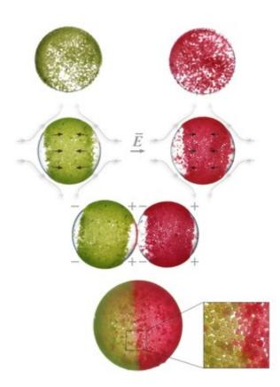
Production of Janus capsules starts with a uniform covering of the surfaces of two drops, each with particles of different properties. After an electric field is applied, microflows force the particles to move to the drop 'equators'. The areas around the drop poles are electrically charged and the drops attract one another. Two drops electro-coalesce forming a densly packed Janus capsule. Credit: Nat. Commun. 5, 3945 (2014)
