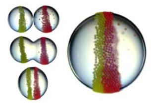
Janus rings resulting from the coalescence of drops containing small amounts of particles. The ring is slightly thicker at the bottom, because the particles sense the Earth's gravity. Credit: Nat. Commun. 5, 3945 (2014)
