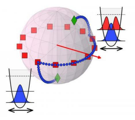
Sphere illustrating the quantum states: The poles represent the two possible vibration states, every other point represents a superposition. The system starts at the south pole, the puls shifts it to the equator, the second pulse to the north pole. Credit: Vienna University of Technology
