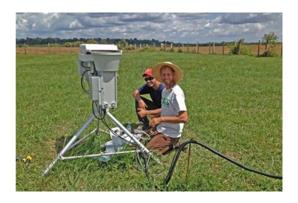
Heath-Powers: Los Alamos scientist Heath Powers, foreground, and on-site technician Vagner Castro work on field equipment for measuring carbon dioxide and water vapor near areas of human habitation in Brazil.
