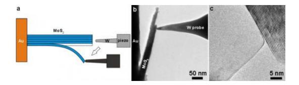
Nanomechanical cleavage of molybdenum disulphide atomic layers. (left) Schematics of the experimental setup inside HRTEM. (center) TEM image of a sharply etched tungsten nanoprobe in contact with the  $MoS_2$  single crystal deliberately placed with (0002) basal atomic planes viewed edge-on. (right) HRTEM image of a cleaved  $MoS_2$  atomic monolayer.
