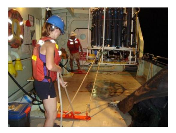
Kelsey Poulson-Ellestad, a former graduate student at the Georgia Institute of Technology, now at Woods Hole Oceanographic Institution, works with a Conductivity, temperature and depth (CTD) sampling rosette, which is lowered over the side of a vessel and is used to collect water samples from various depths. Credit: Kelsey Poulson-Ellestad.
