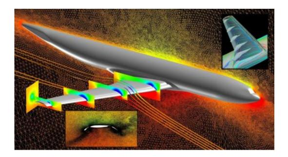
This CFD visualization required a NASA supercomputer to handle the intensive calculations. It shows a mesh adaptation used to simulate a transport aircraft in a high-lift configuration. Credit: NASA / Elizabeth Lee-Rausch, Michael Park
