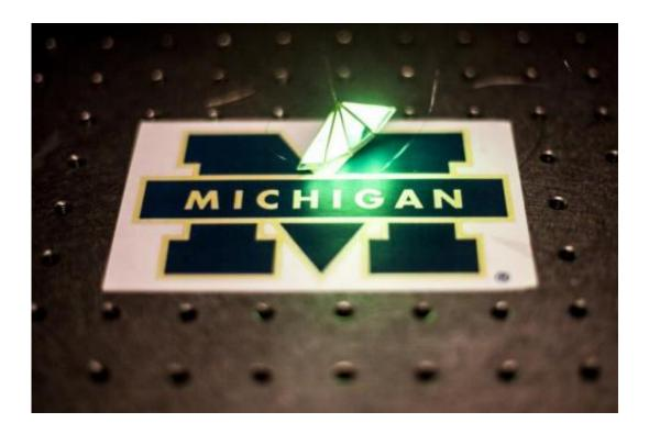
A light concentrating LED in the EECS Building on May 29, 2014. The LED is able to both generate and emit light through its pyramidal shape, enabling for efficient energy use. Credit: Joseph Xu, Michigan Engineering Communications & Marketing
