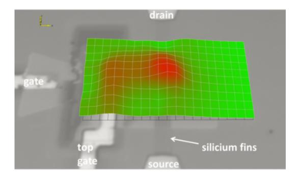
Top view of the upward movement of a piezo FET with 5 parallel silicon bars (also referred to as 'fins') as a result of the piezo-electric effect. When an electrical current is applied across the piezoelectric material, the green parts do not move, but the red ones do.
