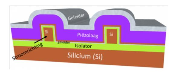
Sketch of the transistor prototype. The transistor current flows through tiny silicon bars, which are enveloped by a package of conductor layers and piezo-electric material. The conductors control the amount of mechanical tension, and also the quantity of electrons in the silicon. In this way, the power can be turned on and off.
