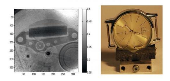
A wristwatch was one of the first items imaged by the new proton radiography system. At left, the inner workings of the mechanism are visible.
