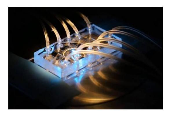
This image shows an example of a rigid epoxy microfluidic device, similar to those used for the new high-throughput system, on an optical microscope. Credit: John Friedah
