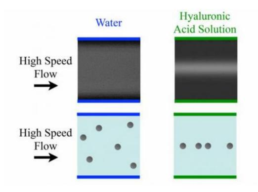
This image shows conventional long-exposure images (top row), and schematically depicted individual particle positions as revealed by the high-speed pulsed-laser imaging technique (bottom row) in a microfluidic device. At high speeds, the focusing effect on particles breaks down in water due to turbulence, whereas the focusing is preserved and enhanced by the team's polymer solution.
