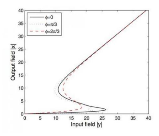
This image shows the input-put field intensity with difference phase  $\phi$  between two components of polarized electric field of the EPF. Credit: World Scientific Publishing, 2014
