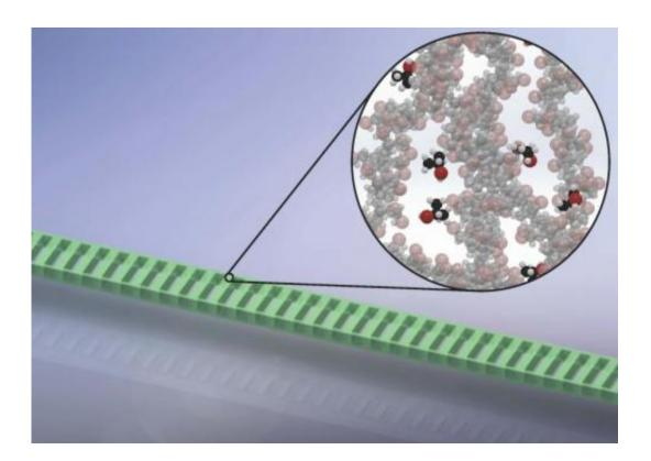
High-sensitivity detection of dilute gases is demonstrated by monitoring the resonance of a suspended polymer nanocavity. The inset shows the target gas molecules (darker) interacting with the polymer material (lighter). This interaction causes the nanocavity to swell, resulting in a shift of its resonance. Credit: H. Clevenson/MIT
