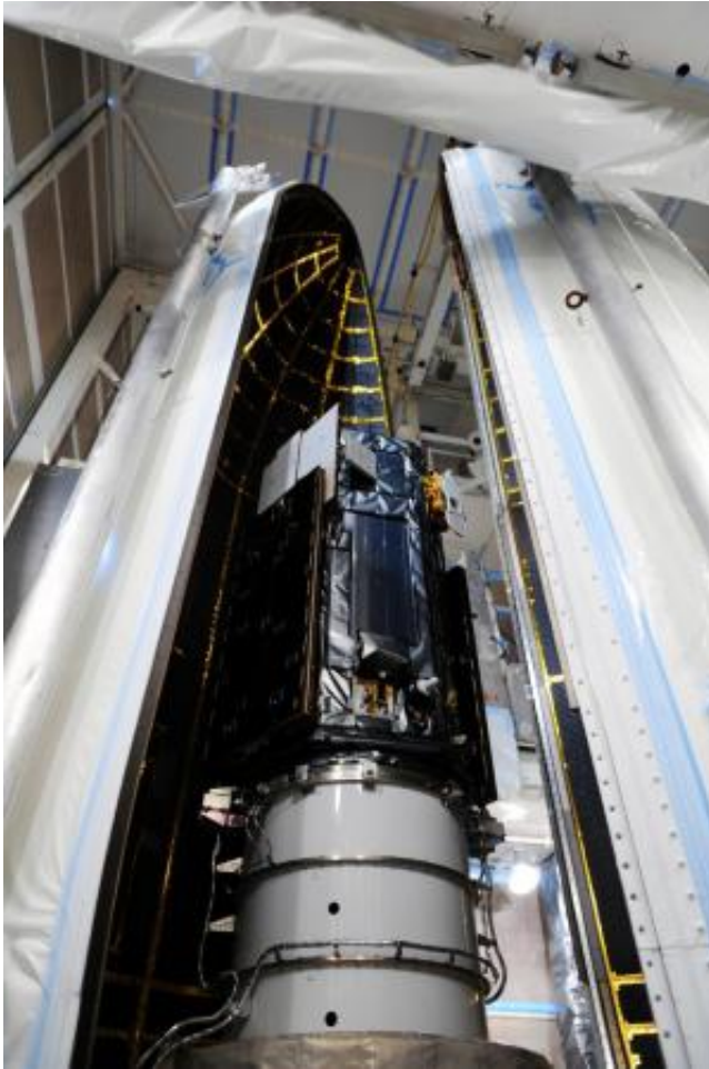
Encapsulation of NASA's Orbiting Carbon Observatory-2, or OCO-2, into the Delta II payload fairing nears completion in the mobile service tower at Space Launch Complex 2 on Vandenberg Air Force Base in California. Credit: NASA/30th Space Wing, U.S. Air Force
