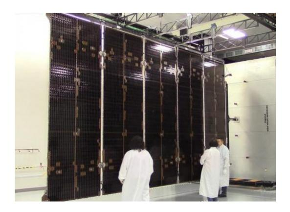
This photo shows a successful deployment of the GOES-R satellite solar array in a Lockheed Martin clean room in Sunnyvale, California, on May 13, 2014. Credit: Lockheed Martin
