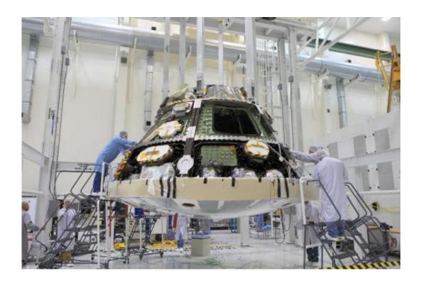
Engineers completed installing the heat shield on NASA's Orion spacecraft ahead of its first trip to space in December. The flight test will send an uncrewed Orion 3,600 miles into space before returning it to Earth for the splashdown in the Pacific Ocean. The heat shield will help protect the Orion crew vehicle from temperatures of about 4,000 degrees Fahrenheit during its reentry into Earth's atmosphere. Credit: NASA/Daniel Casper
