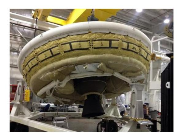
This undated image provided by NASA shows a saucer-shaped test vehicle holding equipment for landing large payloads on Mars in the Missile Assembly Building at the U.S Navy's Pacific Missile Range Facility at Kekaha on the island of Kaua'i in Hawaii. The vehicle, part of the Low Density Supersonic Decelerator project, will test an inflatable decelerator and a parachute at high altitudes and speeds over the Pacific Missile Range scheduled for June 1, 2014. (AP Photo/NASA)
