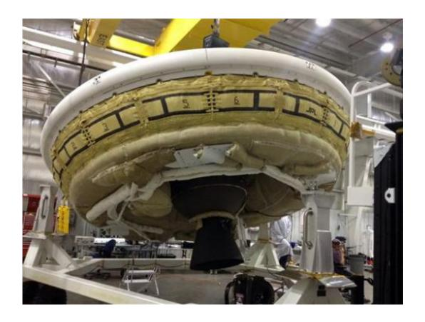
This undated image provided by NASA shows a saucer-shaped test vehicle holding equipment for landing large payloads on Mars in the Missile Assembly Building at the U.S Navy's Pacific Missile Range Facility at Kekaha on the island of Kaua'i in Hawaii. The vehicle, part of the Low Density Supersonic Decelerator project, will test an inflatable decelerator and a parachute at high altitudes and speeds over the Pacific Missile Range scheduled for June 1, 2014. (AP Photo/NASA)
