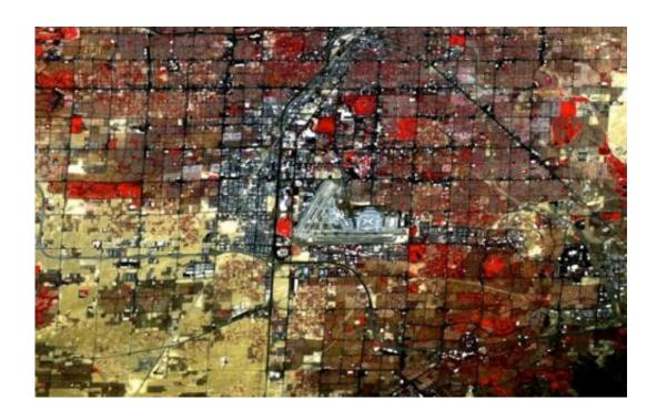
This color infrared composite image is made from three spectral bands of NASA's MASTER instrument mounted on the agency's high-altitude ER-2. The red areas depict green vegetation in Las Vegas on May 30. 2014. Credit: NASA / Dean Neeley / Jeff Myers
