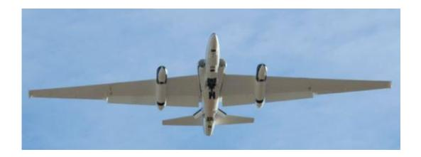
With full flaps and speed brakes deployed, one of NASA's high-altitude ER-2 environmental science aircraft descends on final approach to the runway at Air Force Plant 42 in Palmdale, Calif. The research aircraft is based at NASA
