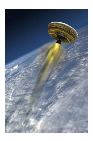
This artist's concept shows the test vehicle for NASA's Low-Density Supersonic Decelerator (LDSD), designed to test landing technologies for future Mars missions. A balloon will lift the vehicle to high altitudes, where a rocket will take it even higher, to the top of the stratosphere, at several times the speed of sound. The Low-Density Supersonic Decelerator Project is managed by JPL for NASA's Space Technology Mission Directorate in Washington. Credit:
