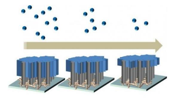
A sample of hygroscopic scaffold made from a forest of carbon nanotubes at Rice University collects and stores water molecules from even arid air. The molecules sink into the forest from the top down, filling up to 80 percent of the scaffold in humid conditions (left), and less in temperate (center) and dry (right) conditions. Credit: Ajayan Group/Rice University
