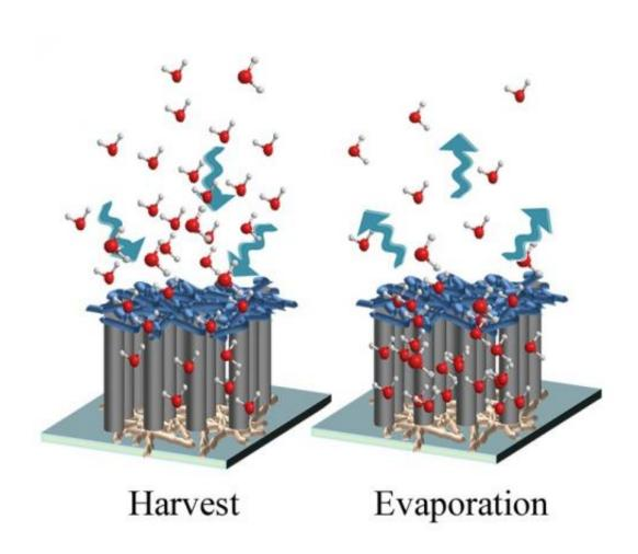
A hygroscopic scaffold created at Rice University is a modified forest of carbon nanotubes that have the ability to harvest water molecules from the air. The water is stored until released either by squeezing the reusable scaffold or until it slowly evaporates back into the atmosphere. Credit: Ajayan Group/Rice University
