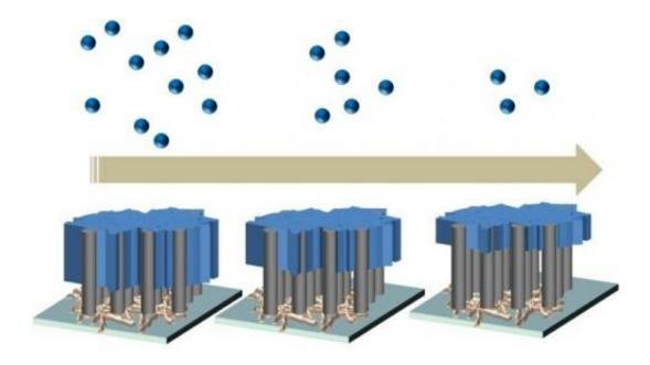
A sample of hygroscopic scaffold made from a forest of carbon nanotubes at Rice University collects and stores water molecules from even arid air. The molecules sink into the forest from the top down, filling up to 80 percent of the scaffold in humid conditions (left), and less in temperate (center) and dry (right) conditions. Credit: Ajayan Group/Rice University
