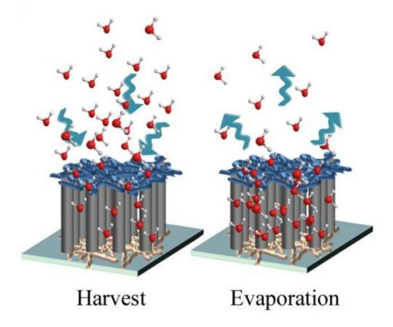
A hygroscopic scaffold created at Rice University is a modified forest of carbon nanotubes that have the ability to harvest water molecules from the air. The water is stored until released either by squeezing the reusable scaffold or until it slowly evaporates back into the atmosphere. Credit: Ajayan Group/Rice University
