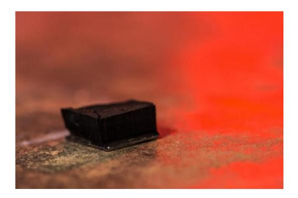
A treated forest of nanotubes can harvest water from arid air, according to researchers at Rice University. The small block, which contains millions of carbon nanotubes, can be altered with hydrophilic and hydrophobic polymers that turn it into a cup that attracts and contains water molecules until they are needed. Credit: Jeff Fitlow/Rice University
