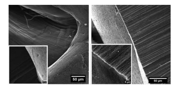
Electron microscope images show the superhydrophobic (water-repelling) side (left) of a hygroscopic scaffold created at Rice University. The image at right shows the hydrophilic (water-loving) side. Credit: Ajayan Group/Rice University
