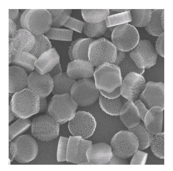
Silicon mesoporous particles, aka SiMPS, about 1,000 nanometers across contain thousands of much smaller particles of iron oxide. The SiMPs can be
