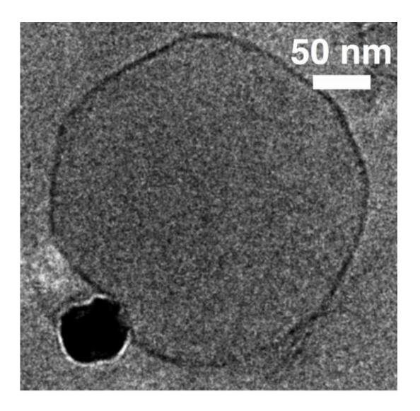
A transmission electron microscopy image of an iron oxide nanoparticle (black) binding to an oppositely charged model cell membrane (phospholipid bilayer). The membrane is in the form of a spherical vesicle dispersed in water. Adhesion between the nanoparticle and the membrane drive the deformation of the vesicle
