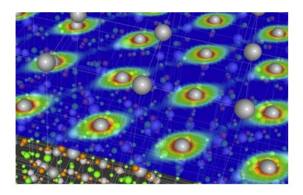
Gray spheres are uranium atoms, around which the electronic state exhibits ellipsoidal anisotropy, being different on the left and right diagonals, breaking fourfold symmetry in the basal plane (blue). (c) 2014 Takasada Shibauchi.
