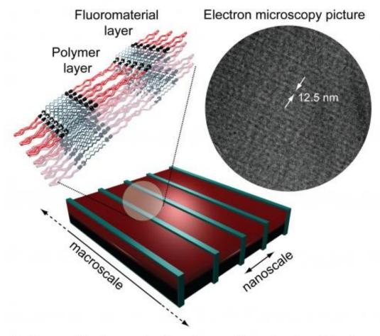
Self-assembled nanostructure keeps aligned up to millimeters
