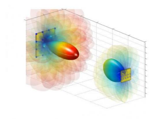
This is a snapshot of millimeter wave dynamic beamforming. The algorithm selects the best beam pattern at both the base station and mobile terminal. Credit: University of Bristol Communication Systems and Networks research group
