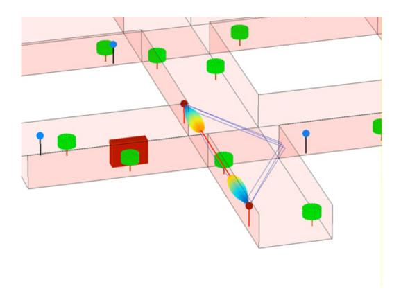
This is a dynamic simulation of a gigabit point-to-point link showing robust operation to a passing bus. Credit: University of Bristol Communication Systems and Networks research group
