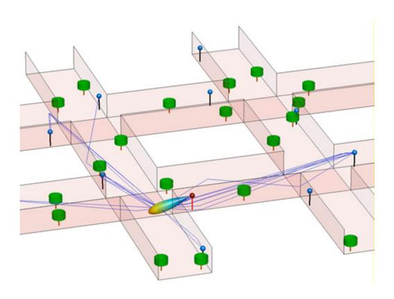
This is a dynamic simulation of gigabit 5G mobile access with lamp post mounted base stations tracking users as they walk around the streets. Credit: University of Bristol Communication Systems and Networks research group
