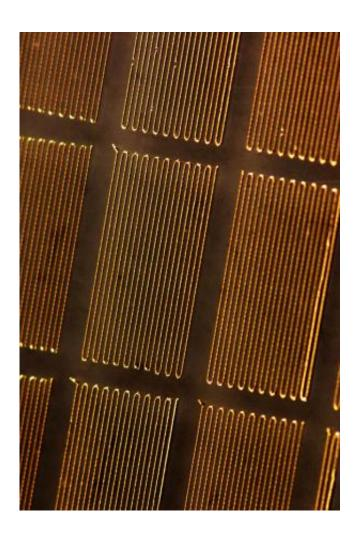
Purdue researchers have developed a technique to embed a liquid-alloy pattern inside a rubber-like polymer to form a network of sensors. The approach might be used to produce "soft machines" made of elastic materials and liquid metals for potential applications in robotics, medical devices and consumer electronics. Credit: Rebecca Kramer/Purdue University
