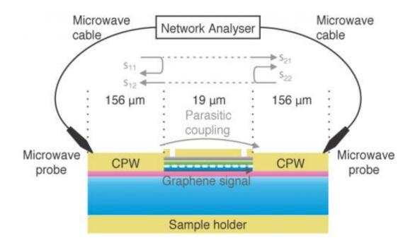
A schematic of the experimental setup is shown. Ham and Yoon measured the change in phase of a microwave signal sent through the graphene. Credit: Hosang Yoon, Harvard SEAS.
