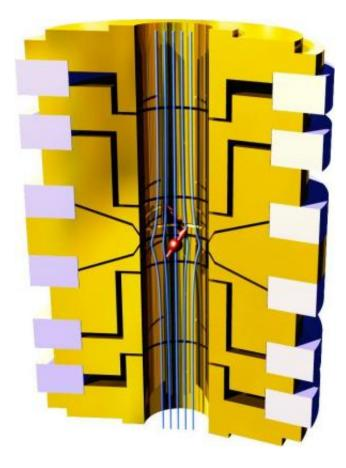
The oscillating proton (red) generates a tiny current which is recorded using highly sensitive electronic detectors. The red arrow represents the magnetic moment of the proton; the green lines indicate the magnetic field in the trap. Credit: Georg Schneider
