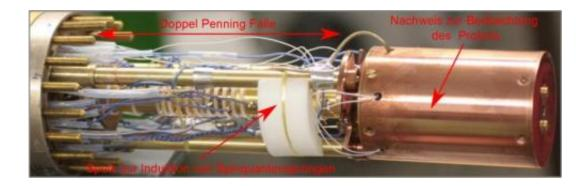
Double Penning trap used to measure the magnetic moment of the proton. The double Penning trap is made of gold-plated cylindrical trap electrodes; the individual trap electrodes are isolated from one another using sapphire rings. During measurements the trap is in an ultra-high vacuum. To the right of the image is the outer housing of a detection instrument which allows for the observation of single protons. The entire structure is about 20 centimeters long. Credit: Andreas Moser
