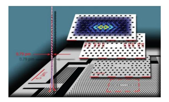
The top layer shows a simulation of the nanostructure confining the light in the tiny red regions. The second layer is the design generated by an approach that mimics evolutionary biology. The bottom two layers show electron micrographs of the realized nanostructure in silicon. The sharp peak on the left is the trace of the long trapping of light. Credit: Fabio Badolato
