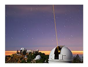
The Lick Observatory's Laser Guide Star forms a beam of glowing atmospheric sodium ions. This helps astronomers account for distortions caused by the Earth's atmosphere so they can see further and more clearly into space. Credit: Laurie Hatch/lauriehatch.com
