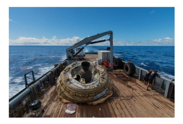
The first "flown" test vehicle of Low-Density Supersonic Decelerator project relaxes aboard the recovery vessel Kahana. During the June 28, 2014, engineering flight, the saucer-shaped test vehicle climbed to over 180,000 feet (about 55,000 meters) in altitude and went as fast as four times the speed of sound. Credit: NASA/JPL-Caltech
