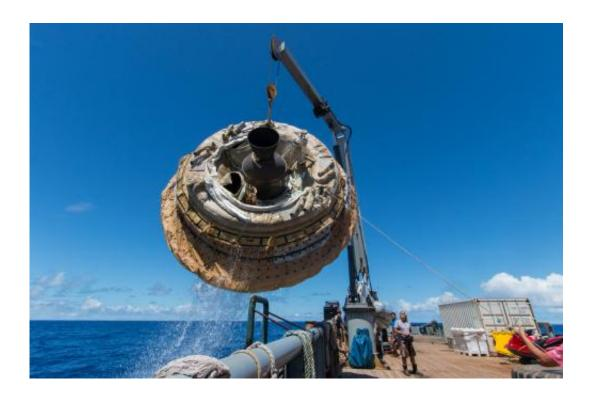
Hours after the June 28, 2014, test of NASA's Low-Density Supersonic Decelerator over the U.S. Navy's Pacific Missile Range, the saucer-shaped test vehicle is lifted aboard the Kahana recovery vessel. Credit: NASA/JPL-Caltech
