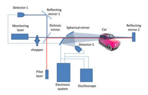
The experiment setup involves two lasers (a monitoring laser and a pilot laser), two detectors, two reflecting mirrors, a chopper, a spherical mirror, a dichroic mirror
