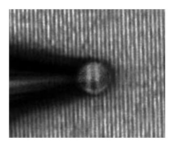
A microsphere connected to the end of a pipette enables sub-diffraction-limit imaging. Credit: L. A. Krivitsky et al.
