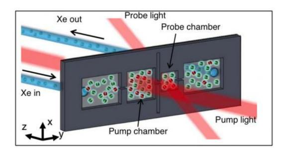
In this experimental set-up, unpolarized xenon gas goes in and hyperpolarized xenon gas emerges from a microfluidic chip when the gas becomes polarized through spin exchange with optically pumped rubidium atoms in the chip.
