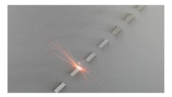
Direct metal laser melting (DMLM) machine in action: A laser fuses metal powder to form one of many successive layers that will form the final manufactured part.
