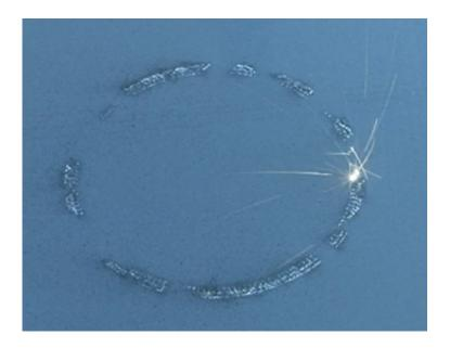
A cylinder is built using Selective Laser Melting (SLM) -- an additive manufacturing process -- and the island scanning pattern, where the region to be melted is divided into smaller islands that are scanned randomly by the laser.
