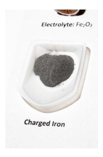
Researchers have created molten air batteries using iron, carbon and vanadium boride because of their ability to transfer multiple electrons. These batteries can store three, four and 11 electrons per molecule respectively, giving them 20 to 50 times the storage capacity of a lithium battery, which can only store one electron per molecule of lithium. Credit: William Atkins, the George Washington University
