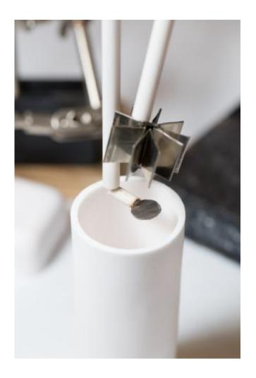
A molten air battery configuration: The air electrode (circle, left) and the metal electrode (right) are lowered into the crucible (white cup), then covered with electrolyte, which is then heated until it is molten. Molten air batteries have the highest intrinsic electric energy storage capacities of any other batteries to date. Credit: William Atkins, the George Washington University
