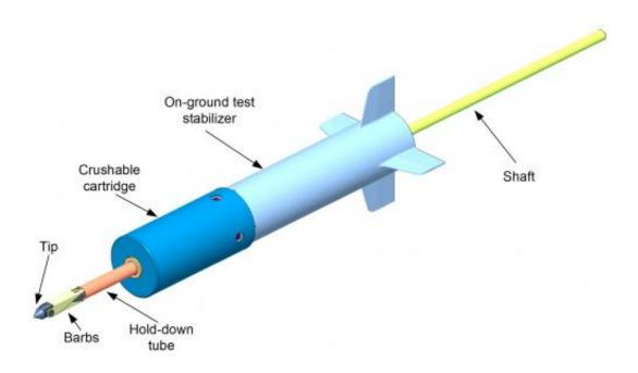
Airbus Defence and Space's preliminary design for a space harpoon system, incorporating a penetrating tip, crushable cartridge to help embed it in the target satellite structure and barbs to keep it sticking in so the satellite can then be
