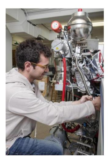
This is the ead author on the Caltech paper, Daniel Stolper, introducing a sample of methane into the mass spectrometer. Credit: Caltech
