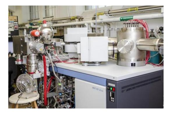
The Thermo IRMS 253 Ultra is Caltech's prototype mass spectrometer, which enables John Eiler and his team to determine formation temperatures for methane samples. Credit: Caltech
