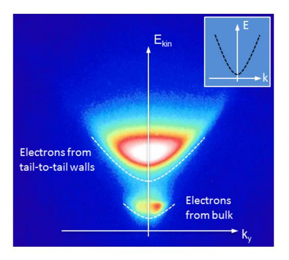
The kinetic energy distribution of emitted photoelectrons when a sample is illuminated with X-rays at 641.2 eV. Electrons emitted at domain walls with enhanced electronic conduction in ErMnO3 travel with more kinetic energy, giving the walls a distinct appearance in X-PEEM images. Credit: *Applied Physics Letters/* Jakob Schaab, et. al.
