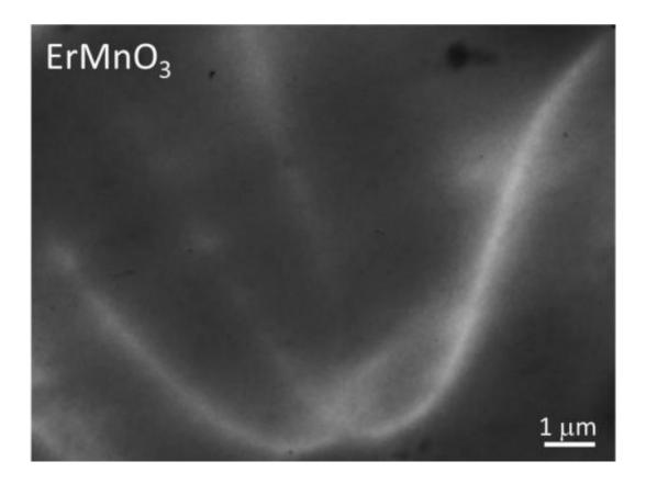
An X-PEEM image shows conducting domain walls in ErMnO3, which appear brighter than the surrounding bulk material. Credit: Applied Physics Letters/ Jakob Schaab, et. al.
