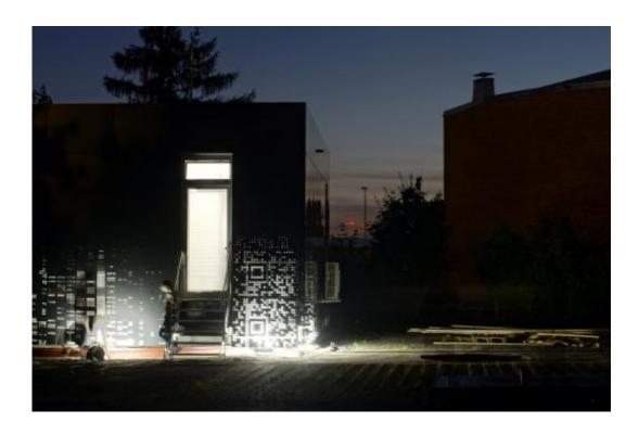
LOBSTER at night: The front is made of aluminum composite boards milled in a computer-supported manner. Credit: Robin Nagel/Moritz Karl
